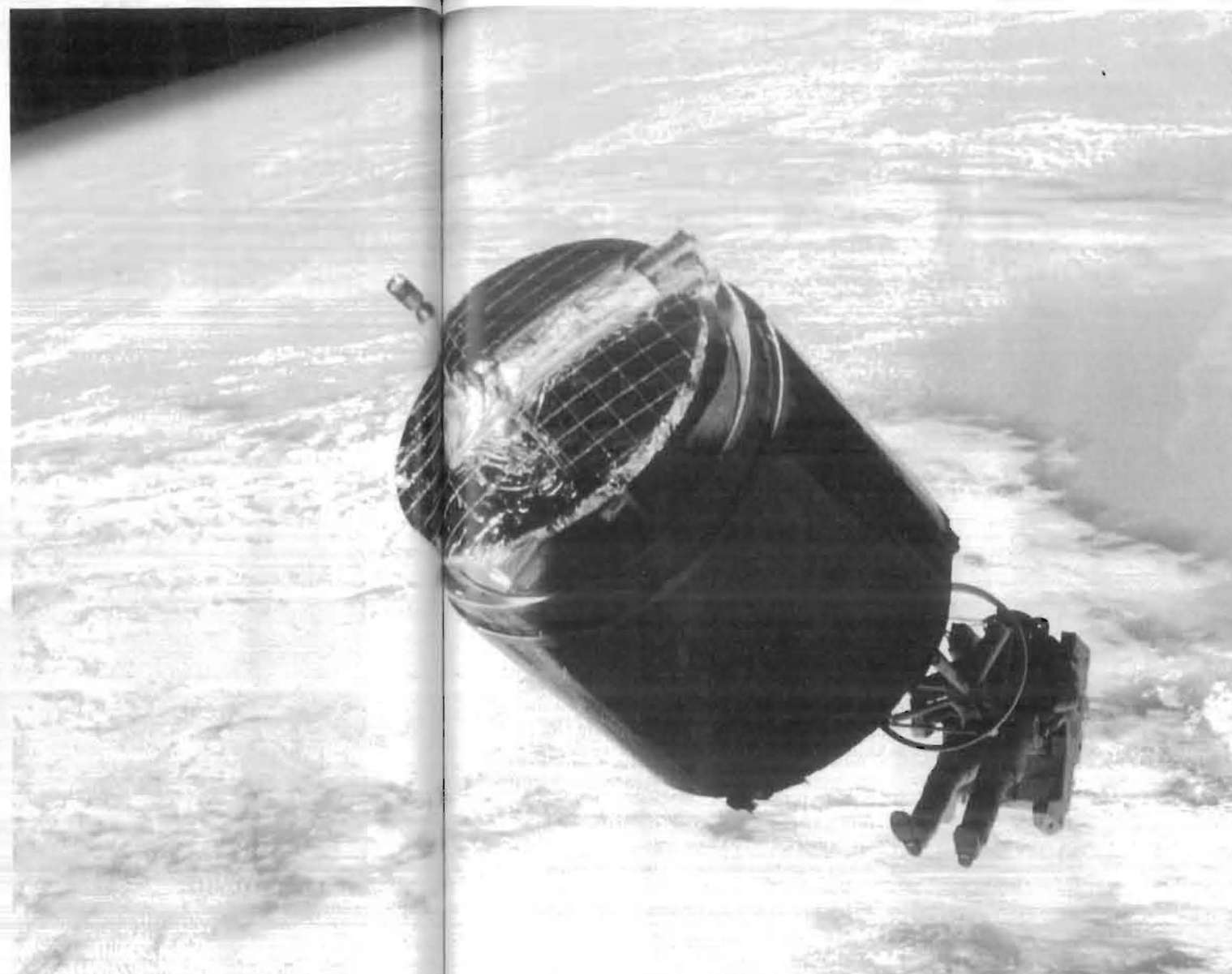
Left: Astronaut Dale Gardner uses a manned maneuvering unit—also known as the Buck Rogers backpack—which enables him to move about in space via jets of air and to dock with a spinning Westar VI satellite. He soon pulled the satellite into the shuttle's cargo bay.
